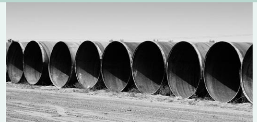
Water pipes are already being manufactured to insert into the San Vicente Pipeline tunnel.
