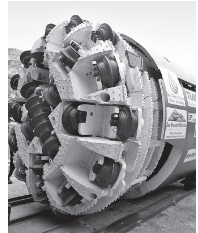
The 12-foot-tall, 400-foot-long main beam machine was delivered to the San Vicente Portal in June.
