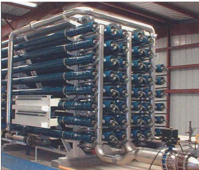
Demineralization of brackish groundwater in Oceanside.
