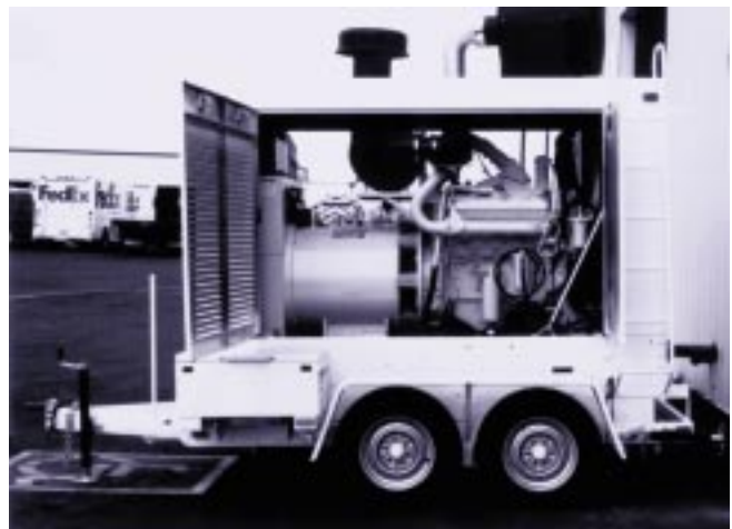
A portable generator used to produce electricity for various purposes such as carnival rides or motion picture lighting.
