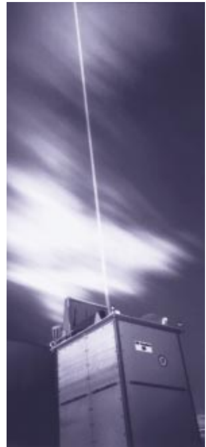
A lidar instrument measures ozone levels aboveground by sending out a laser beam during the Southern California Ozone Study.
