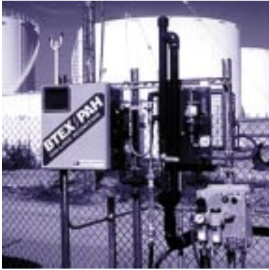
Turner Designs Inc. "TD-4100" online aromatic hydrocarbon monitor, which Cal/EPA certified in May 1997.
