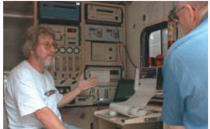
District chemists are able to perform low level oxides of nitrogen (NOx) source tests using equipment housed in a mobile van. NOx contributes to ozone formation.
