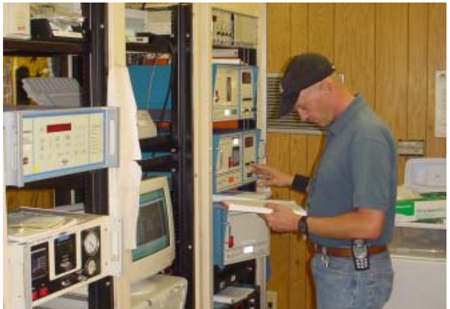
An electronic instrument technician performs routine maintenance on an ozone instrument to ensure its accuracy.
