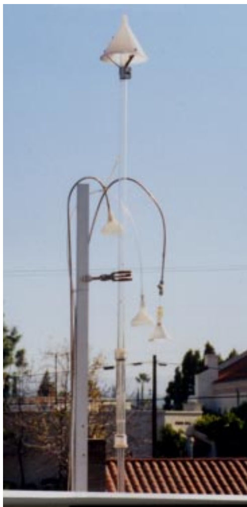
Air is drawn into an ozone monitor by large glass tubes.
